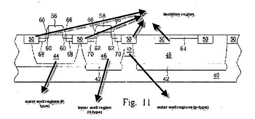
each outer well region has an upper surface which includes a source/drain region 60/62 (col. 4, lines 57-67); a field effect transistor having at least a p-type gate conductor 58 located above the inner P-well region; and wherein the outer N-well regions 46/48 and the inner P-well region 52 are in contact with the subcollector (col. 4, line 67 to col. 5, line 6 and FIG. 11).
